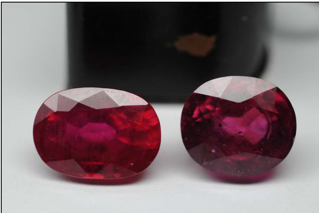
Figure 4: Lead glass filled rubies made with ruby material from “Niassa”, seen in Bangkok in January 2009. Rounded gas bubbles are visible in the stone on the right. Photo: V. Pardieu/GIA Lab Bangkok, February 2009.
