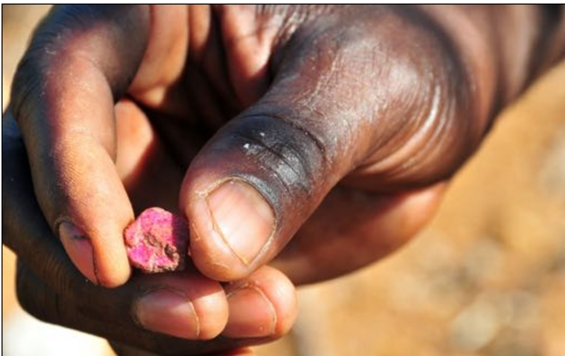
Figure 45: A typical low quality ruby found on the ground of the mining site at Namahaca: the stone fissures are brownish due to the presence of limonite and the stone shows some abrasion typical of secondary deposits. Photo: V. Pardieu / GIA Laboratory Bangkok, December 2009.
