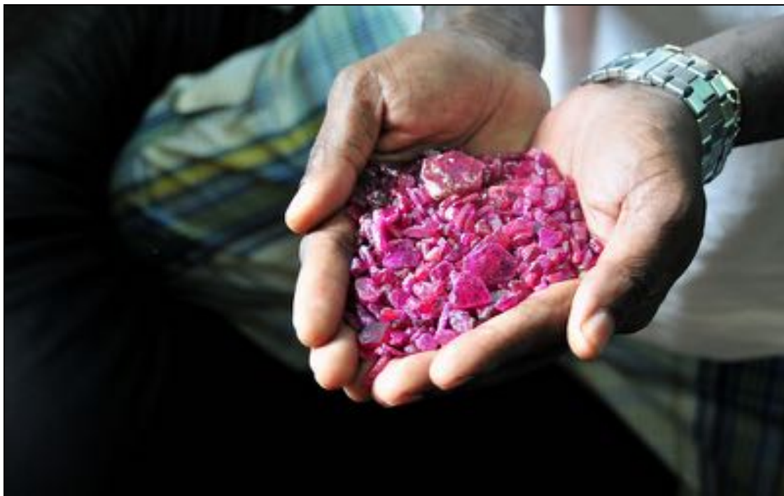
Figure 52: A West African dealer presenting a parcel of "Montepuez" rubies of mixed quality. Most of the material is suitable for lead glass type treatment as if the color is fine the stones are heavily fractured. Photo: V. Pardieu / GIA Laboratory Bangkok, November 2009
