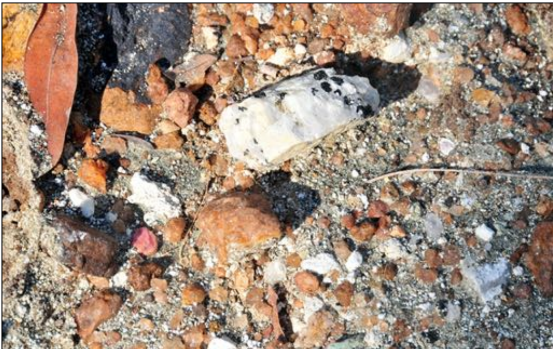
Figure 49: On the ground, near the primary deposit, the rocks are different from those seen by the party near the stream. Whilst quartz is still present we also found a lot of feldspar and what looks to be black tourmaline. Photo: V. Pardieu / GIA Laboratory Bangkok, December 2009.
