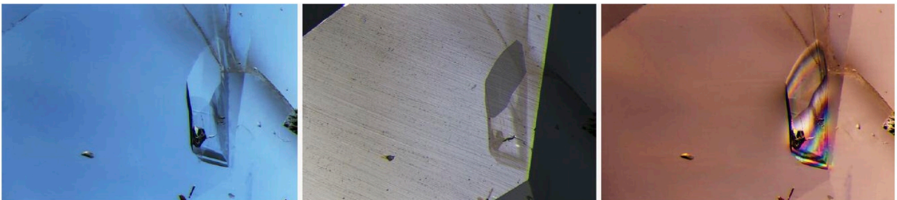
Figure 6. A colorless grandidierite crystal was seen in a sapphire examined by author EBH at Lotus Gemology in Bangkok (left). In reflected light, the grandidierite inclusion showed a duller luster than the sapphire host (center) and cross-polarized light revealed birefringent interference colors (right). Photomicrographs by E. Billie Hughes; field of view 1.7 mm.
