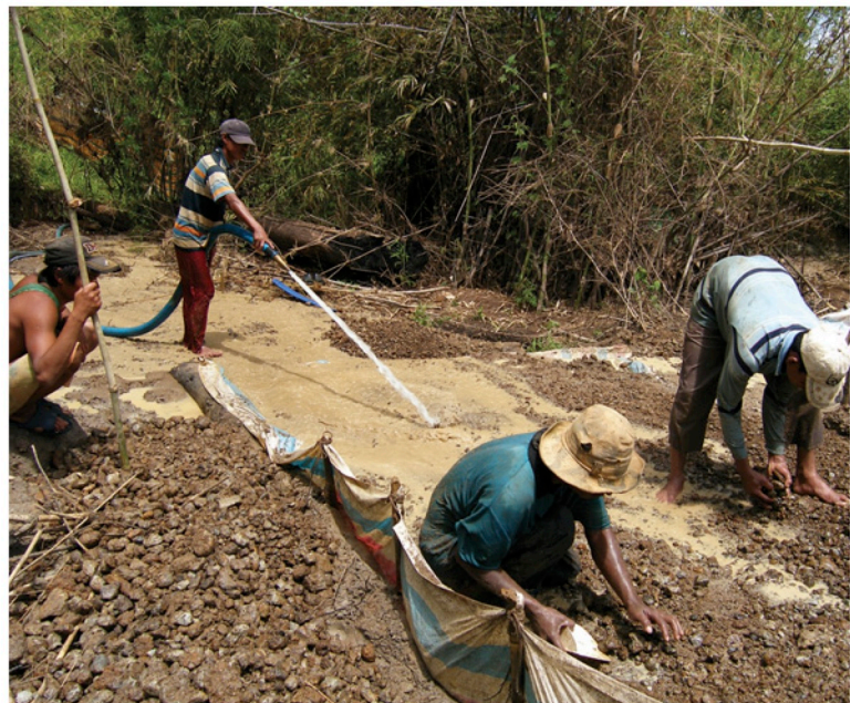
Figure 24. The best-known Cambodian zircon deposit is at Bo Keo (left), where there are ~30 active mines. The shafts in this region are typically about 15 m deep. At Bo Kalap (below), there are ~10 active pits; the excavated material contains basalt cobbles and requires washing to recover the zircon. Photos by M. H. Smith.
