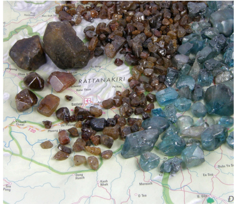
Figure 23. These rough zircons were recovered from Ratanakiri Province, Cambodia. The blue rough (up to 7 g) was produced by heating brown stones such as those on the left (up to 24 g). Photo by Prasit Prachagool.
