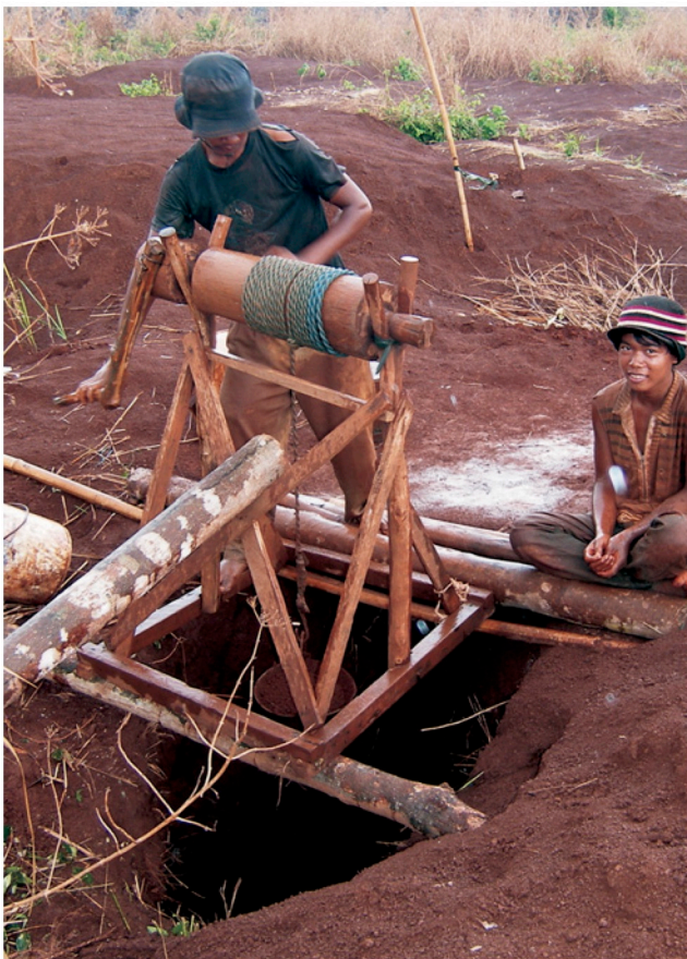
Figure 24. The best-known Cambodian zircon deposit is at Bo Keo (left), where there are ~30 active mines. The shafts in this region are typically about 15 m deep. At Bo Kalap (below), there are ~10 active pits; the excavated material contains basalt cobbles and requires washing to recover the zircon. Photos by M. H. Smith.
