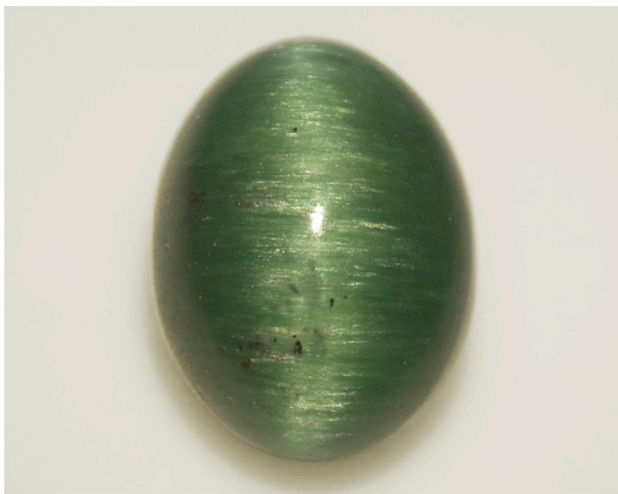
Figure 21. This bluish green cat's-eye cabochon (36.63 ct) proved to be serpentine. Photo by G. Choudhary.
