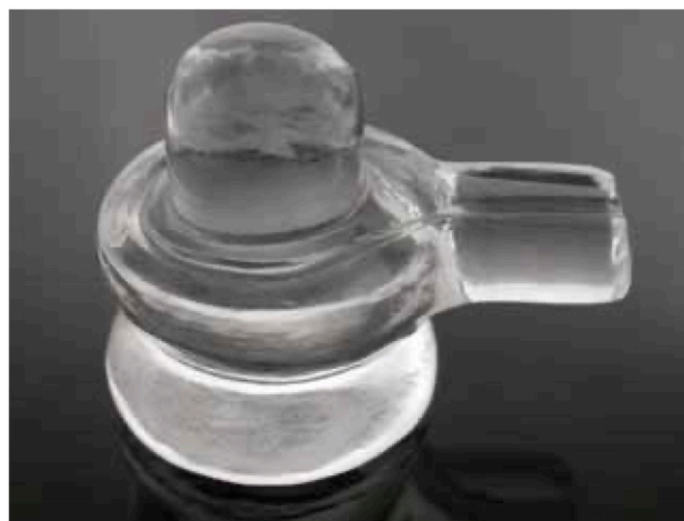
Figure 22. This 188 ct "Shivling," approximately 4.0 cm tall, was represented as rock crystal quartz, but proved to be manufactured glass. Photo by G. Choudhary.
